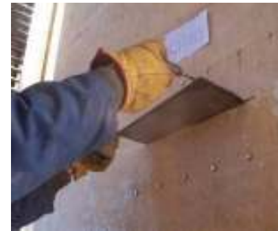
Single flat-jack test (detection of state of stress) carried out at the Monza Tower (Binda, 1998)
